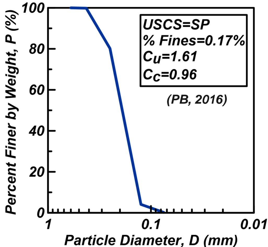
Values obtained using the ASTM D422 - 63 method. The selected values are the average value from 2 tests.
