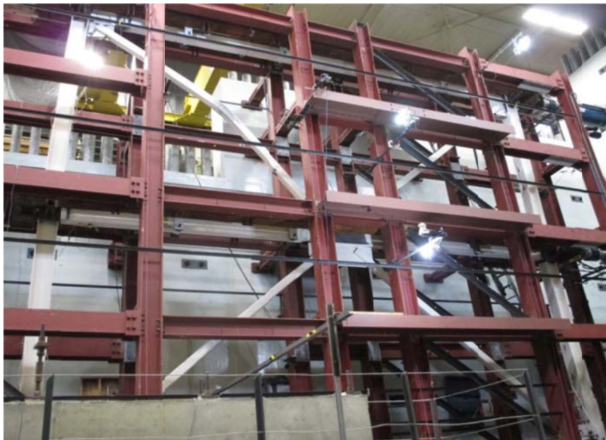
Above: The split-X OCBF at 2% roof drift. Buckling of the brace can be seen in the upper left bay.
