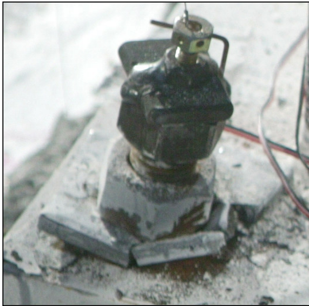
Figure 3.26 – Fracture of top plate washer of Test #6
