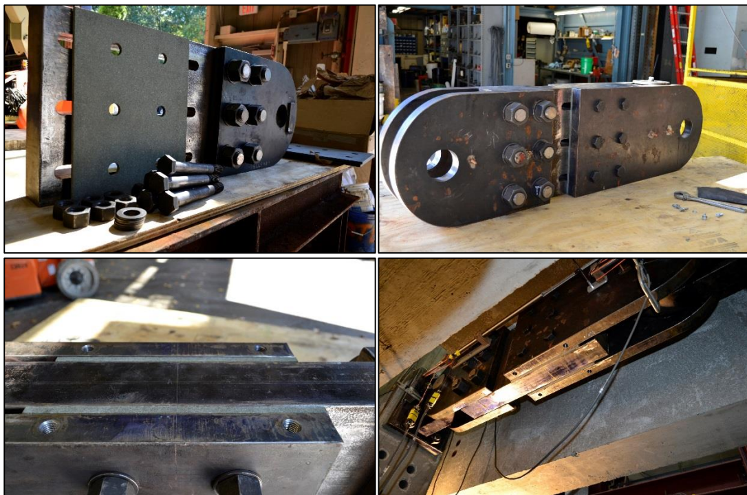
Figure 4.101: Components, assembly and installed FD in phase II-3
