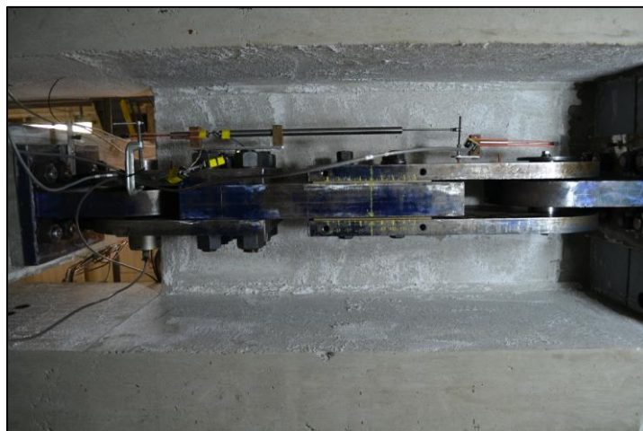
Figure 4.60: Installed FD on the specimen for phase II-1
