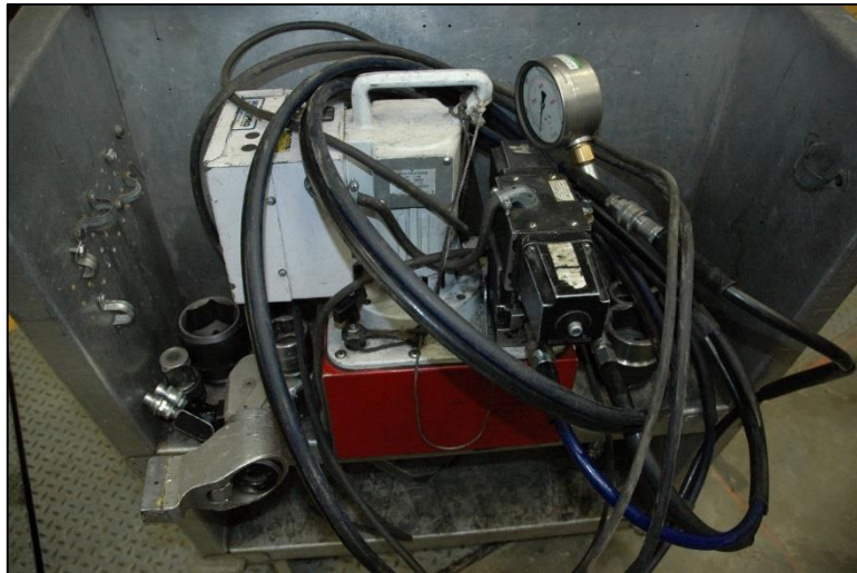
Figure 4.74: Hydraulic gun used for the bolt pretensioning
