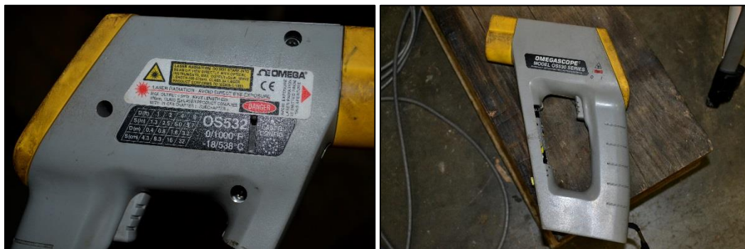
Figure 4.75: Infrared gun used to measure the surface temperature of the internal steel plate
