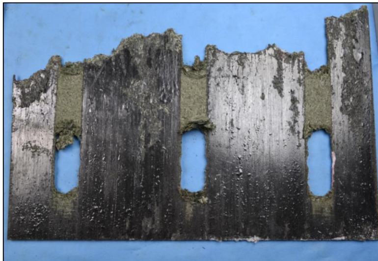
Figure 4.98: Fractured West RF42 friction plate at the end of phase II-2
