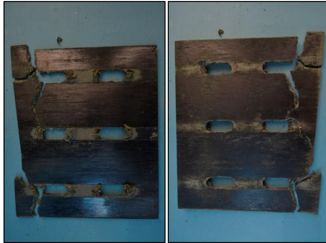
Figure 4.123: Fractured West RF42 friction plate at the end of phase II-3
