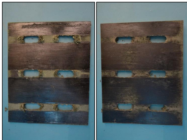
Figure 4.122: East RF42 friction plate with elongated bolt holes at the end of phase II-3
