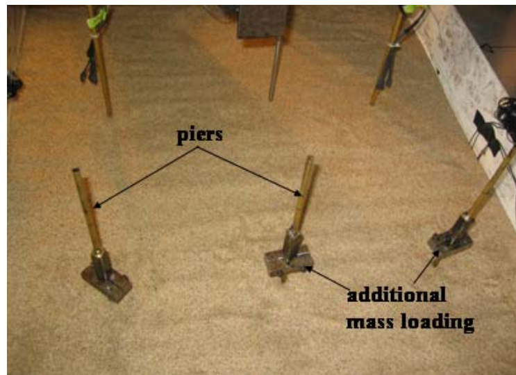
Figure 4.2 Extra weights added to increase the moving rate
