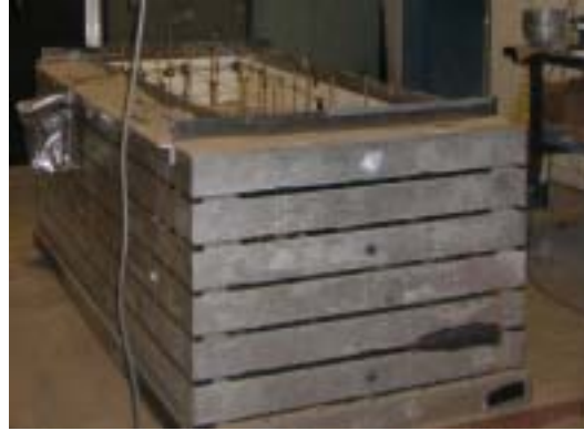
Figure 3.2 Flexible Shear Beam (FSB1) soil container
