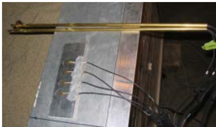
Figure 3.6 Photo of strain gauges' Wheatstone half bridge connection
