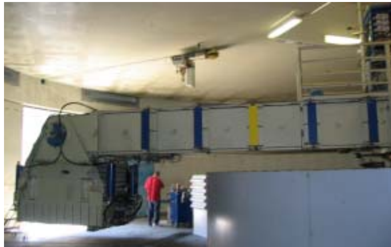
Figure 3.1 The 9-m radius geotechnical centrifuge at UC Davis
