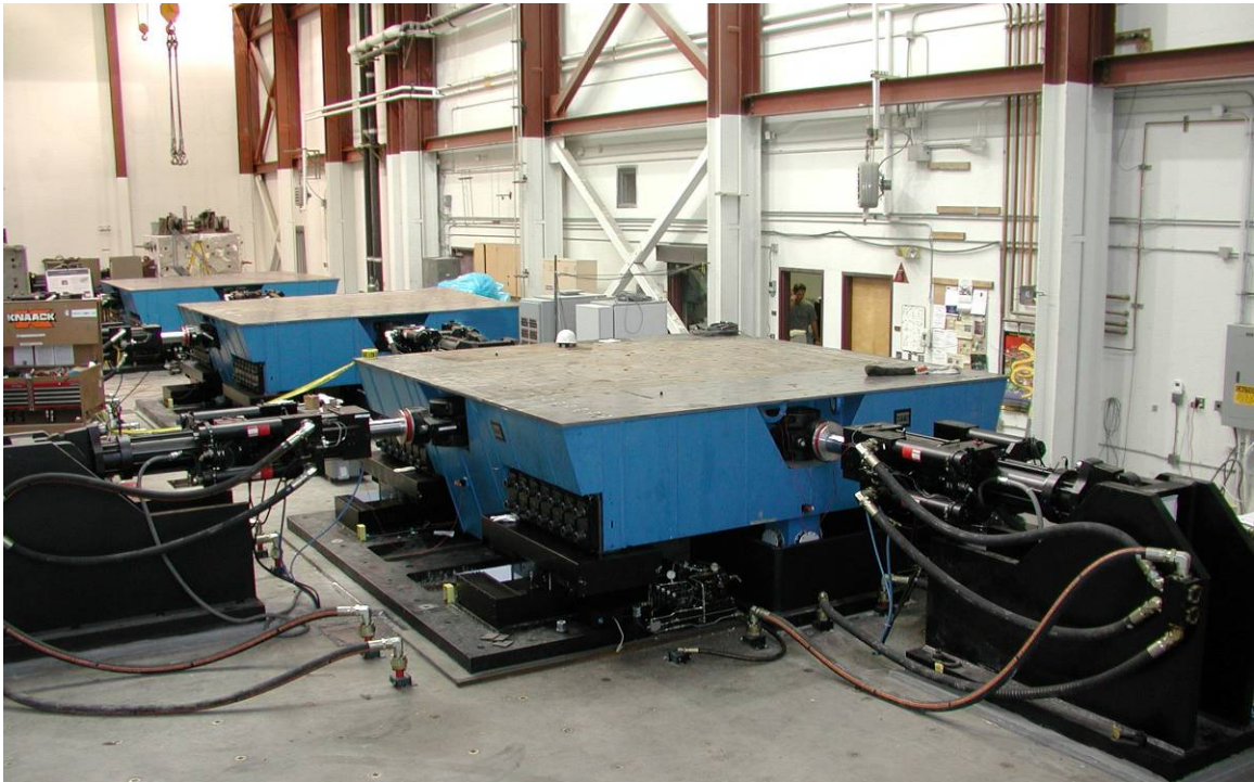
Figure 5-24: Bare shake tables prior to assembly of bridge.
