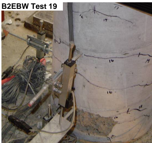
Figure 6-12: Photographs of damage progression for bent 2, east column bottom west side, through test 20.
