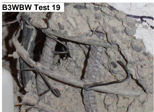
Figure 6-24: Photographs of damage progression for bent 3, west column bottom west side, through test 20.
