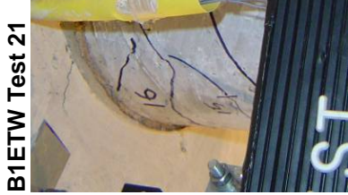
Figure 6-28: Photographs damage progression for bent 1, east column top west side, for tests 20-22.
