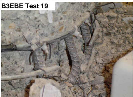
Figure 6-18: Photographs of damage progression for bent 3, east column bottom east side, through test 20.
