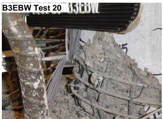
Figure 6-20: Photographs of damage progression for bent 3, east column bottom west side, through test 20.
