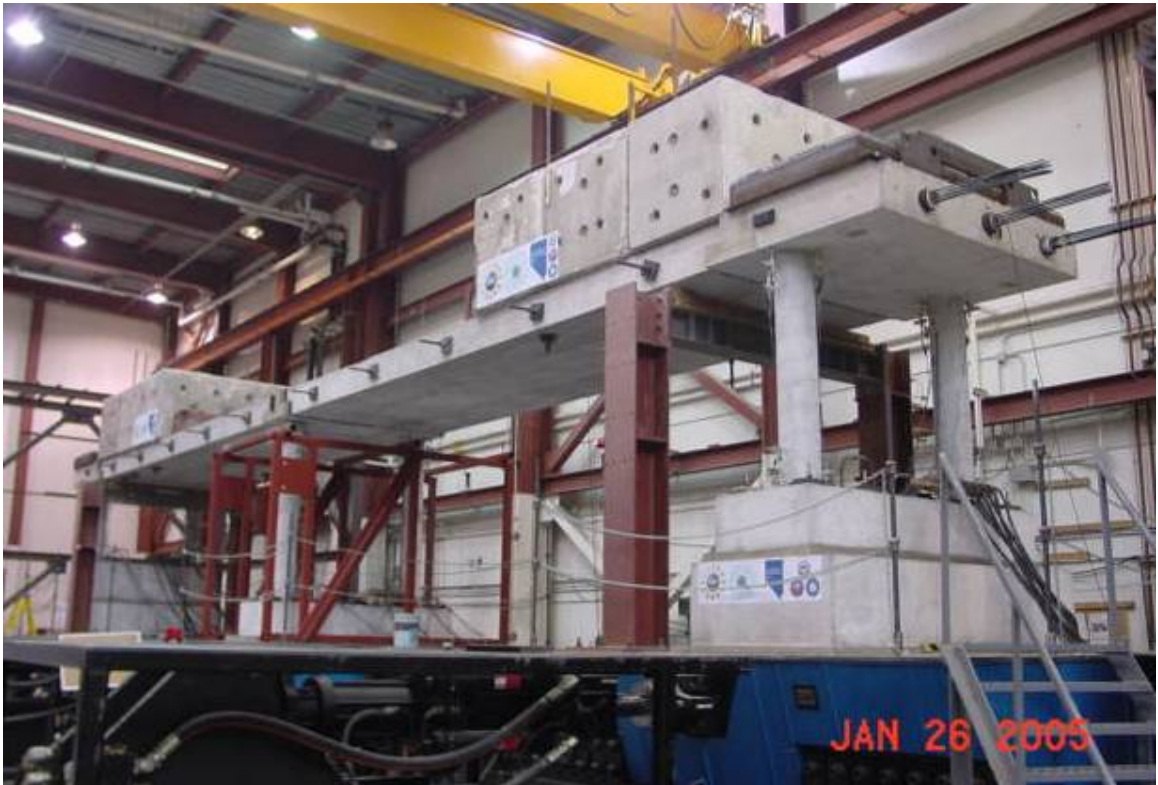
Figure 5-42: Completed bridge before shake table testing.
