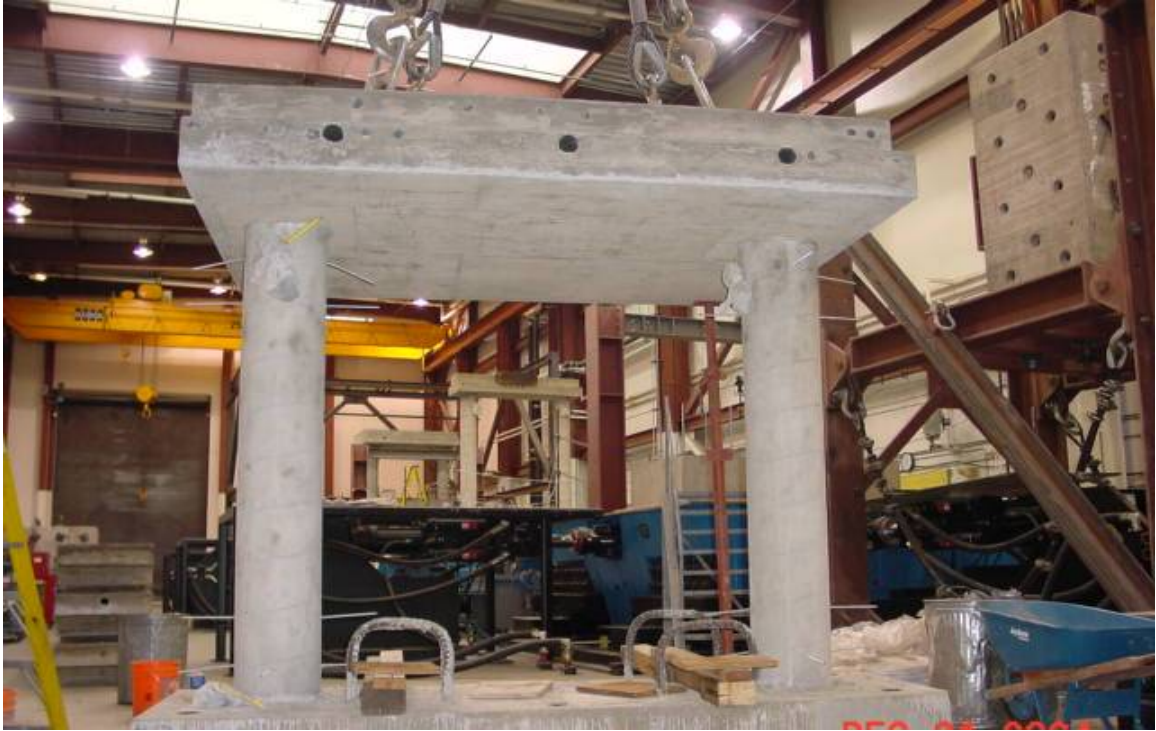
Figure 5-27: Transportation of bents to shake tables using crane in laboratory.
