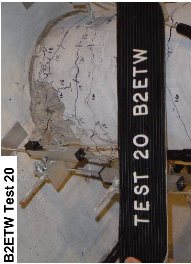
Figure 6-32: Photographs damage progression for bent 2, east column top west side, for tests 20-22.
