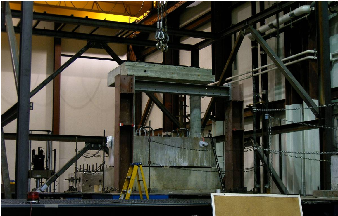
Figure 5-28: Placement of bent 3 on end shake table.
