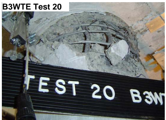
Figure 6-21: Photographs of damage progression for bent 3, west column top east side, through test 20.
