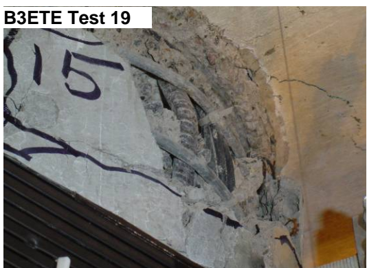
Figure 6-17: Photographs of damage progression for bent 3, east column top east side, through test 20.
