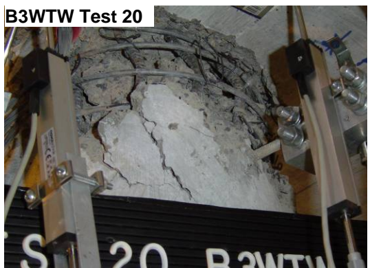
Figure 6-23: Photographs of damage progression for bent 3, west column top west side, through test 20.
