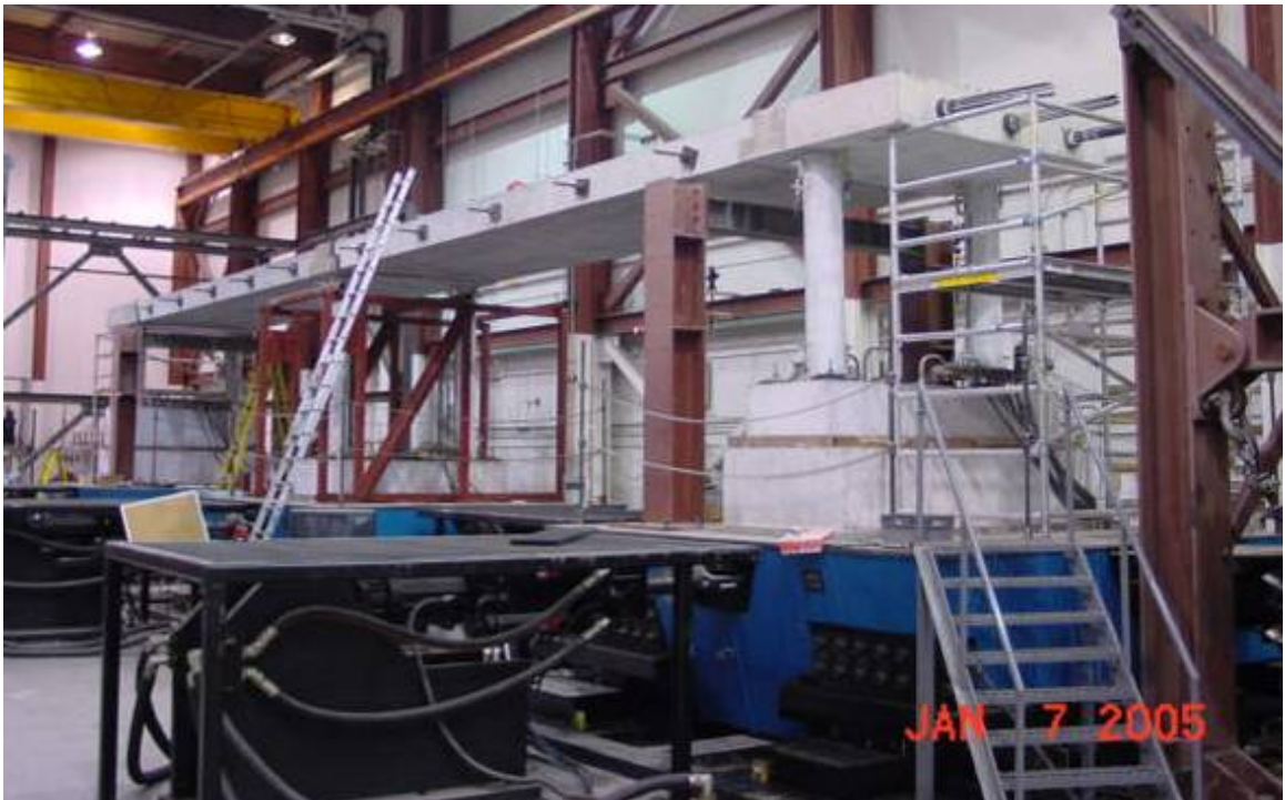
Figure 5-40: Post-tensioned bridge model prior to placement of masses.
