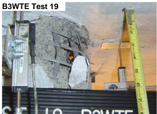
Figure 6-21: Photographs of damage progression for bent 3, west column top east side, through test 20.
