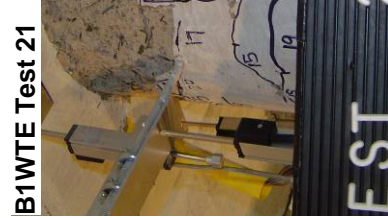
Figure 6-29: Photographs damage progression for bent 1, west column top east side, for tests 20-22.
