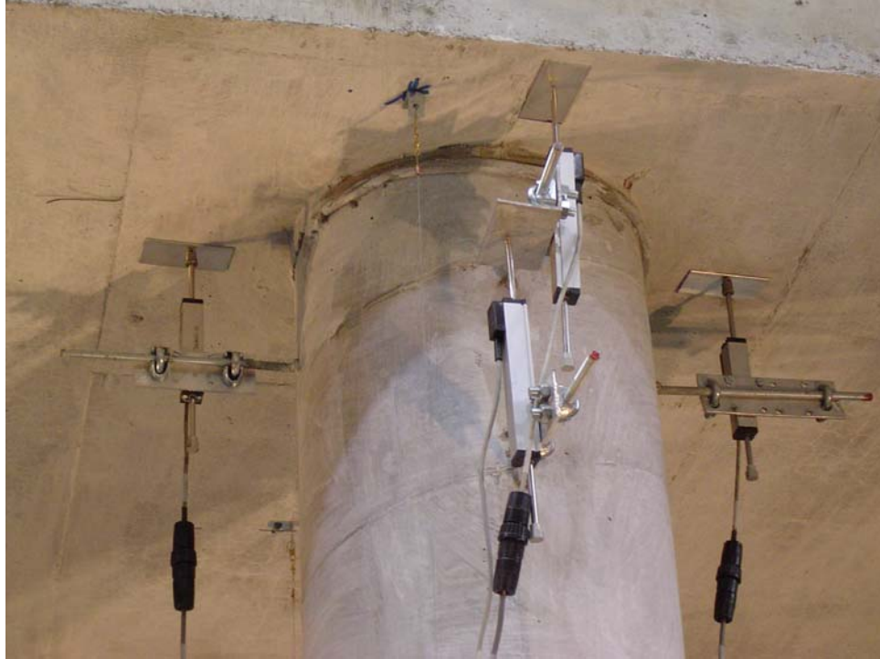
Figure 3-9: Photograph of typical curvature measurement in plastic hinge region.
