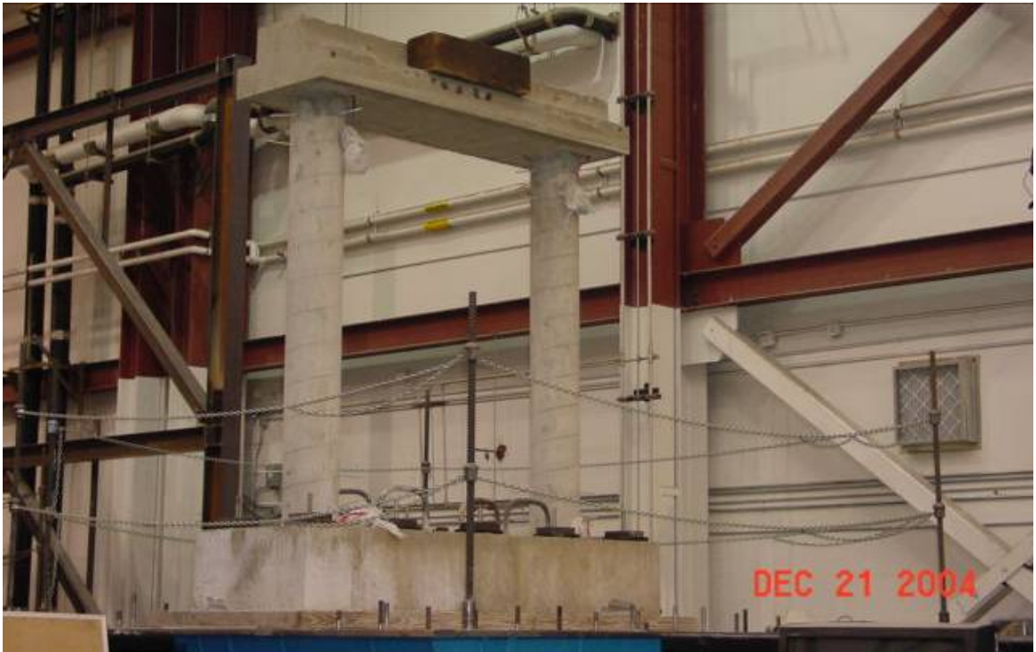
Figure 5-26: Placement and grouting of bent 2 on middle shake table.
