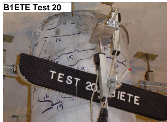
Figure 6-1: Photographs of damage progression for bent 1, east column top east side, through test 20.
