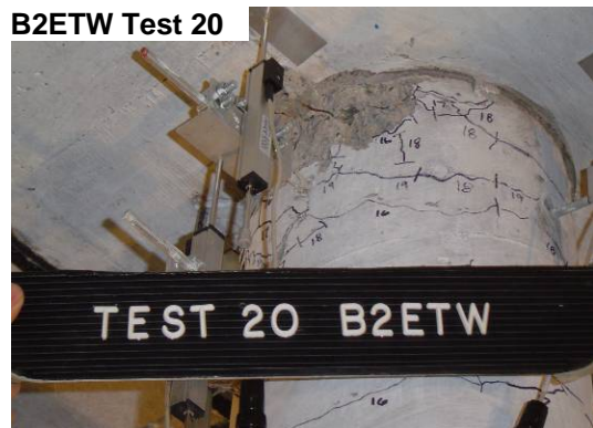
Figure 6-11: Photographs of damage progression for bent 2, east column top west side, through test 20.
