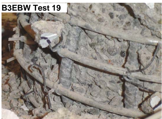
Figure 6-20: Photographs of damage progression for bent 3, east column bottom west side, through test 20.
