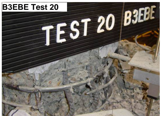
Figure 6-18: Photographs of damage progression for bent 3, east column bottom east side, through test 20.
