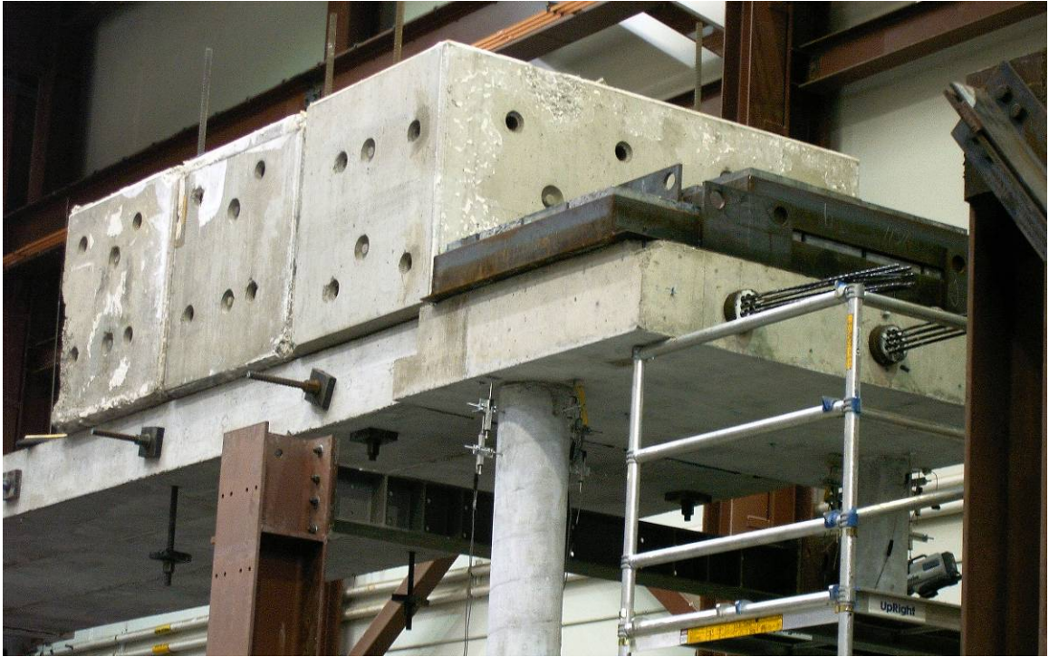
Figure 5-41: Placement of masses on top of bridge superstructure.
