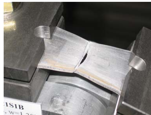
(f) fracture of top plate at \theta_{1.5}=0.36 rad
