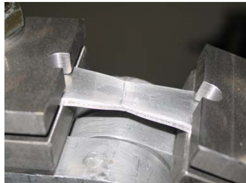
(f) Fracture of top plate at \theta_{1.5''}=0.36\text{rad}
