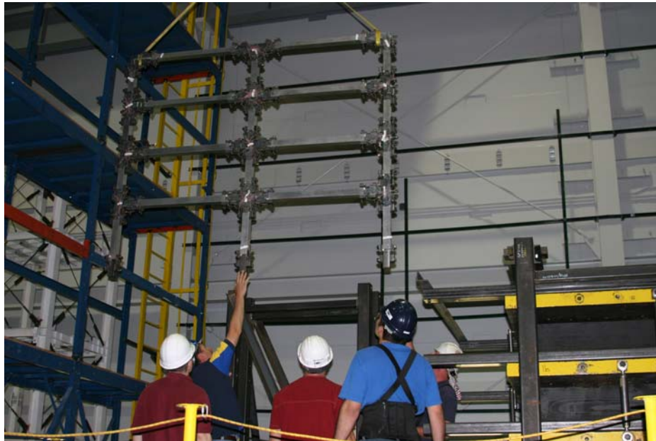
Figure 7.3. Installation of test Frame #1 on the shaking table
