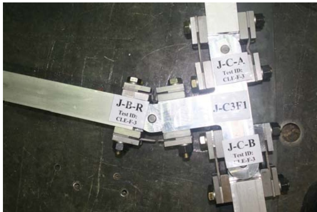
(c) exterior joint of test Frame #2 at the end of collapse test
