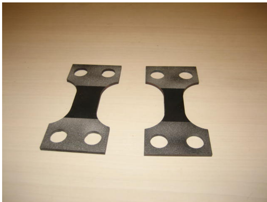
(b) Photo of typical flange plates
