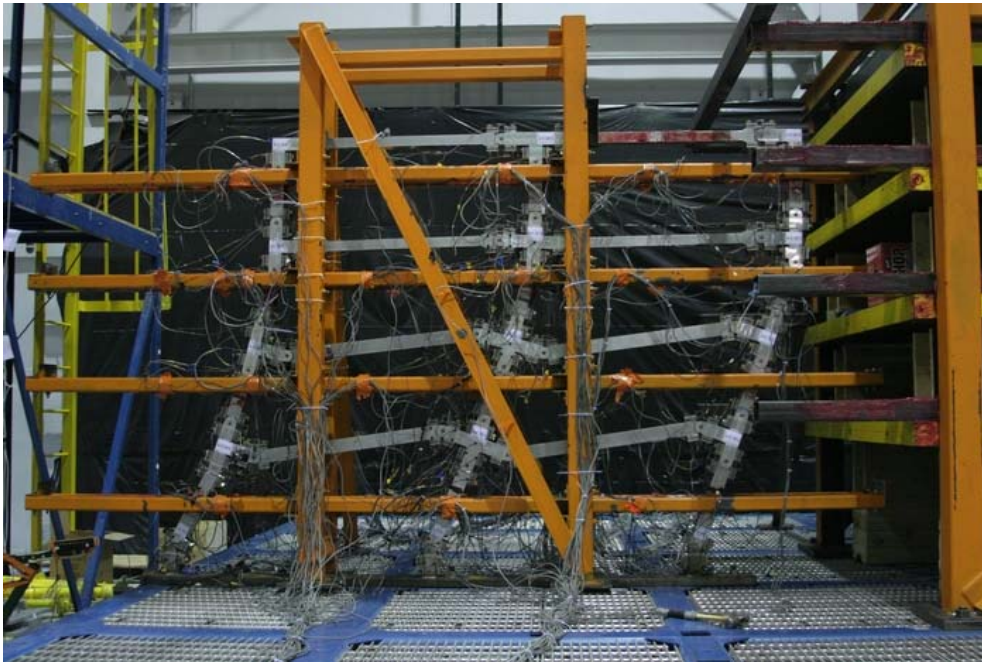
Figure 7.18. Collapse mechanism of Frame #1 after completion of CLEF
