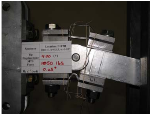
(e) plastic hinge element at \theta_{1.5''}=0.25\text{rad}
