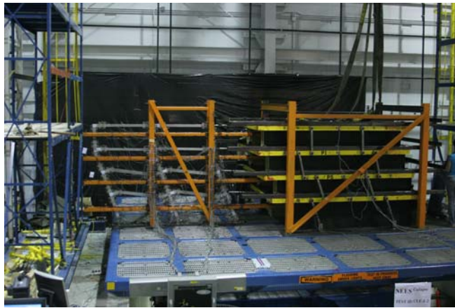
(b) test setup at the end of collapse test (Frame #2)
