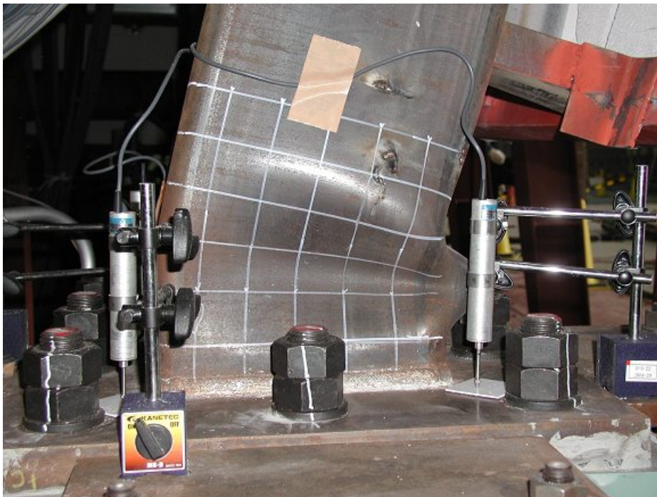
Figure 8.24. Local buckling at the base exterior column after the end of the collapse test (100% Takatori motion)
