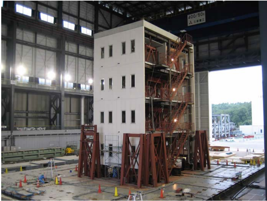
Figure 8.15. E-Defence 4 story building after completion of construction on the shaking table (picture courtesy of Hyogo Earthquake Engineering Research Center)
