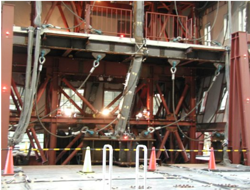
Figure 8.23. First story collapse mechanism of the 4-story structure
