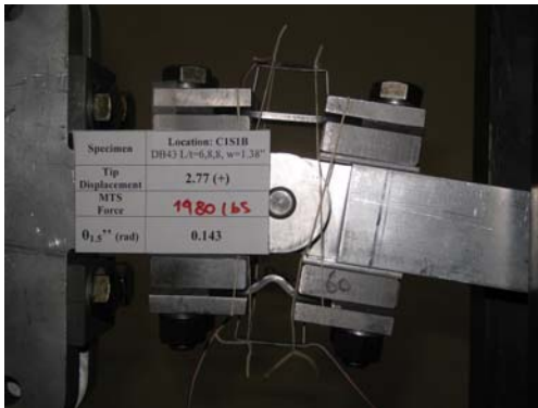
(e) plastic hinge element at \theta_{1.5}=0.14 rad
