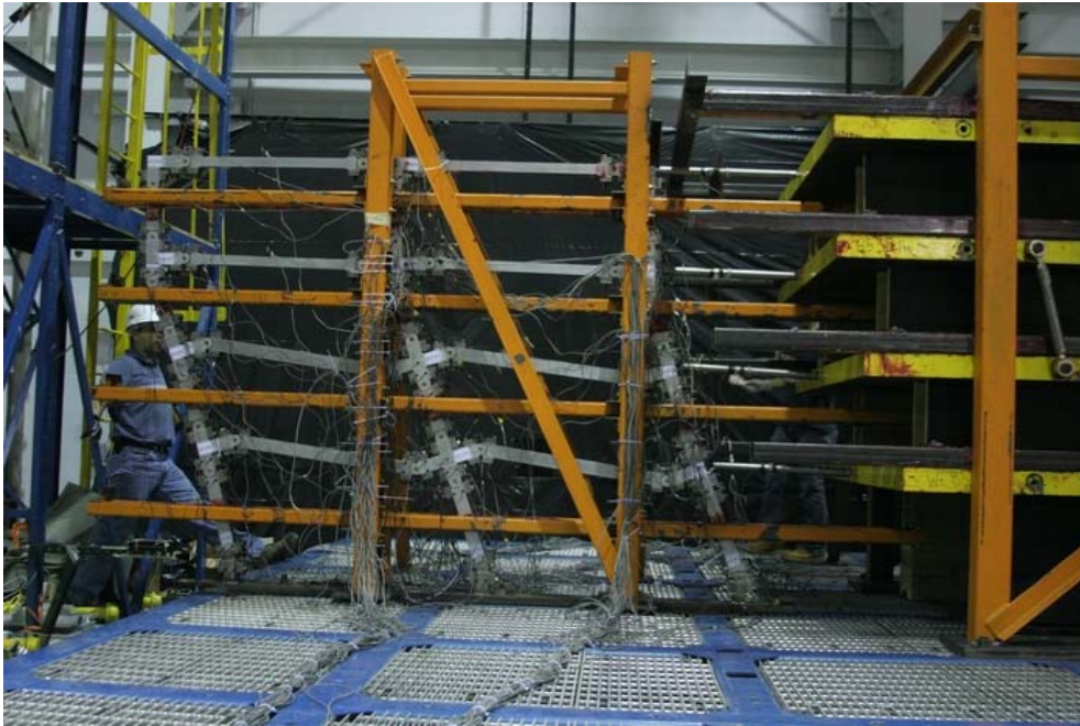
Figure 7.35. Collapse mechanism of Frame #2 after completion of CLEF
