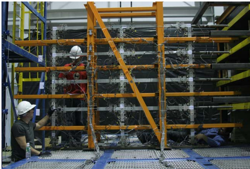
(b) test frame after installation on the shaking table
