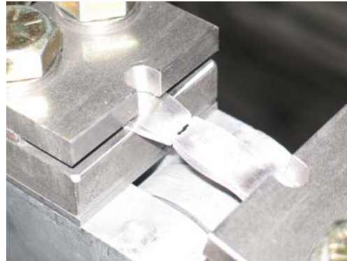
(e) plastic hinge element at \theta_{1.5''}=0.22\text{rad} (f) fracture of top plate at \theta_{1.5''}=0.19\text{rad} (-)
