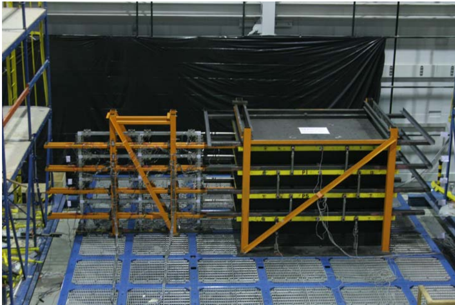
Figure 7.5. Test setup after completion of erection process on the shaking table (Frame #1)
