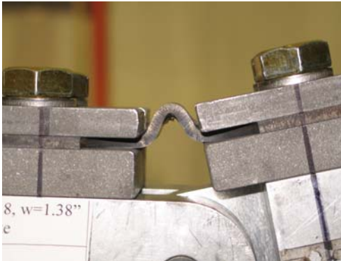
(e) local buckling at \theta_{1.5''}=22.5\text{rad}
